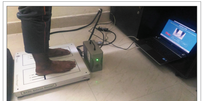
Figure 1: Test in progress on a Balance platform with a Balance screener
