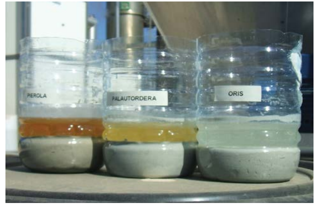
Figure 8: The results obtained from the on-site leachate process for the different leachate under study.
