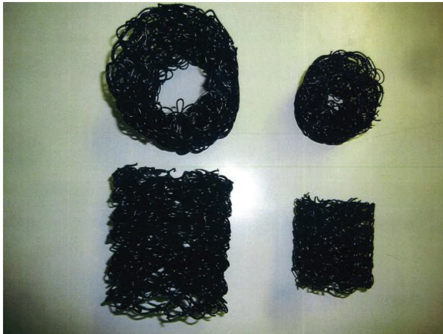
Figure 5: Anaerobic filter media.
